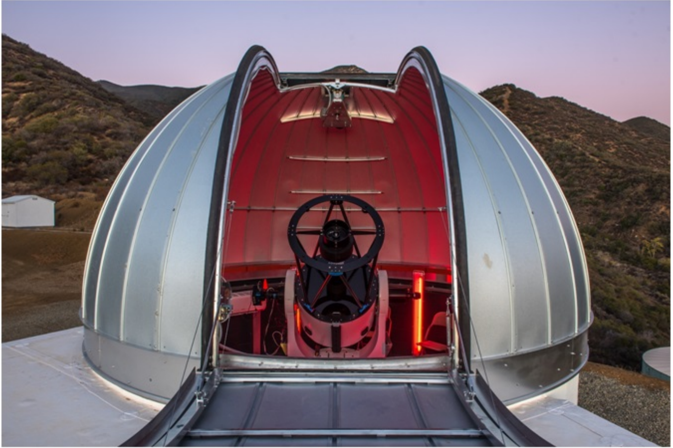
Figure 2. The Thacher Observatory underwent a complete renovation in the fall of 2016, which included installation of a shrink-wrapped and weatherproof roof, a new, fully robotic, Ash Dome, a Plane Wave CDK 700 telescope, and an Andor iKon L-series CCD camera. Photo credit: Paul Gardner, Observatory Systems.
